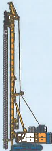
VdW Vor-der-Wand Bohren Front-Of-Wall drilling (FOW)
